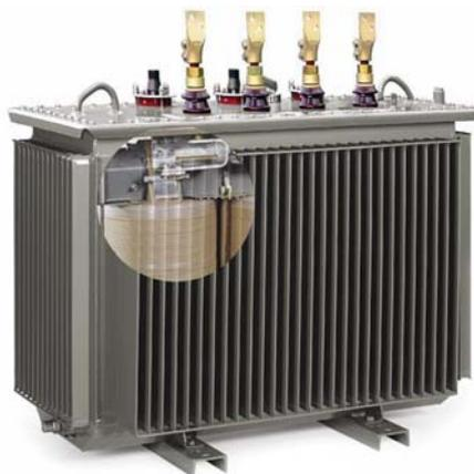
PowerSafe Distribution Transformer with short connections inside and low current densities secures good mechanical strength. IEC60076 -5 result is only 0.45% change in reactance after short-circuit test.
